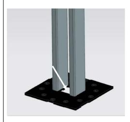
5. Apply the enclosed silicon glue on the top side of the base plate. Take the stainless steel cover plate and move it over the profiles in direction to the base plate. It covers the screw heads.
