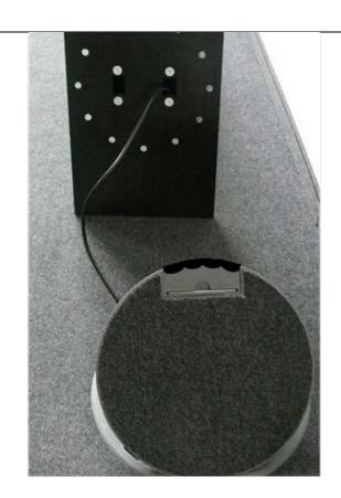
4. Let the cables wired through the base plate hang over the plate.
