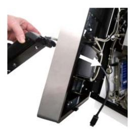
Plug the cable and mount the two screws you removed before to fix the EFT at the housing.
