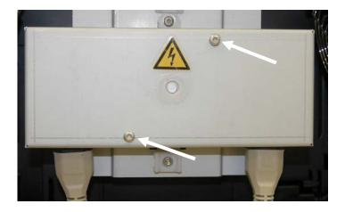
Guide the power cable from above through the cable channel into the power distributor.
