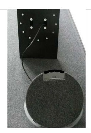
3. Let the cables wired through the base plate hang over the plate.
