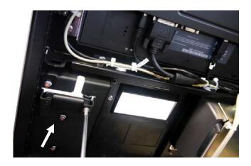
Remove the bracket including the support plate. Loosen the two screws.
